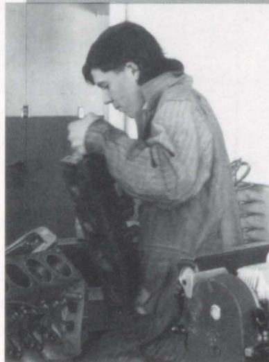
Carter Schiffman lifts a head into place on the engine block. Marc Wooley and J.J. Delong tighten down the rocker arms on this engine.
